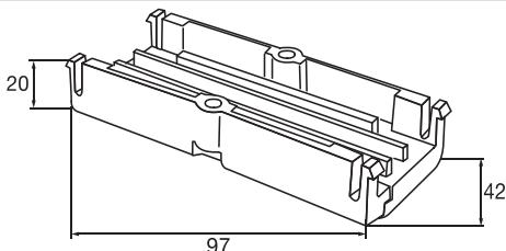
**Stacking protection/spacer for chair frame, for tube diameter 16 mm**
